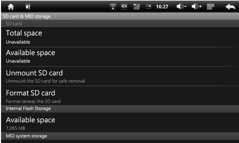
**Notes: pls removing the SD card by the option delete the SD card safely in case of damaging the device by remove it directly.**
